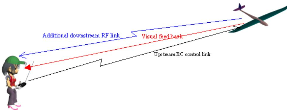
Fig 2 – Improved feed back loop with addition RF link
